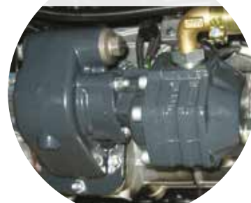
Power take-off connected to the vehicle gearbox
