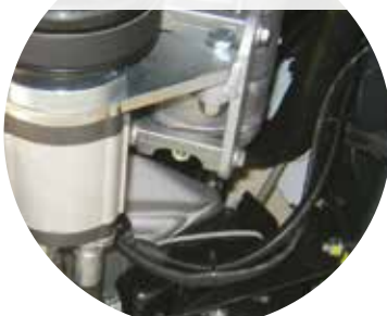
Power take-off with electric clutch
