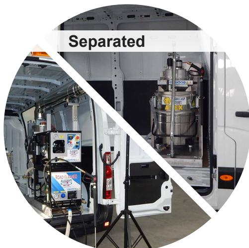
The separated installation helps approach the restoration site with the rear of the vehicle, thus facilitating the ascent and the descent of the operators from the vehicles through the two doors. The distribution of the weight is improved, since the water tank is located in the central part, while the operating unit is in the rear one. The remaining part of the loading compartment can be used for the storing of equipment and various accessories.
