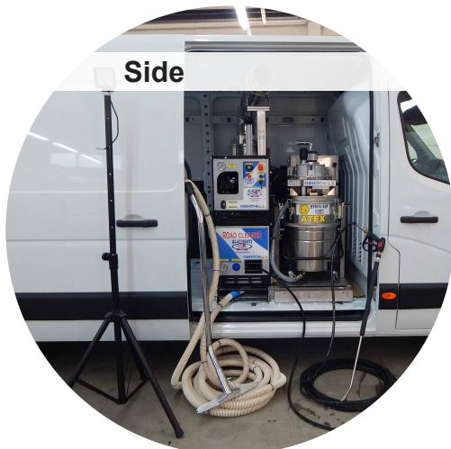
The lateral installation of the system helps approach the restoration site with the side of the vehicle, besides centrally distributing the weight of the system. Thus, there is enough space in the rear part of the loading compartment for the transport of equipment and various accessories.
