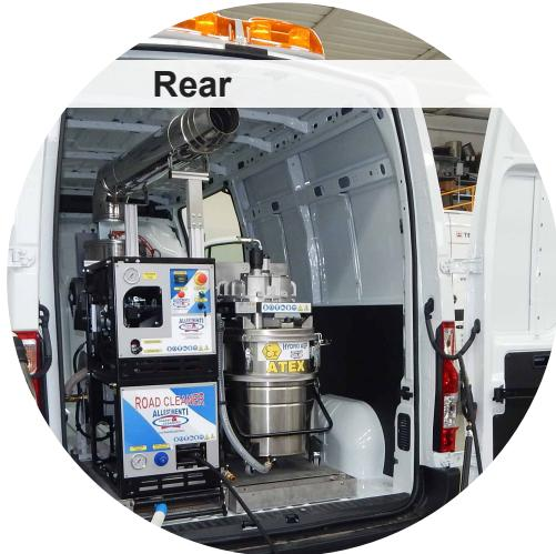
The installation of the system on the rear part helps approach the restoration site with the rear of the vehicle, thus letting enough space in the front of the loading compartment for equipment and various accessories.
